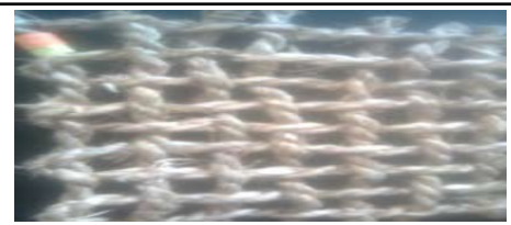
Fig.8: 10 mm thick paddy straw Geomesh with 12x12 mm aperture size.
