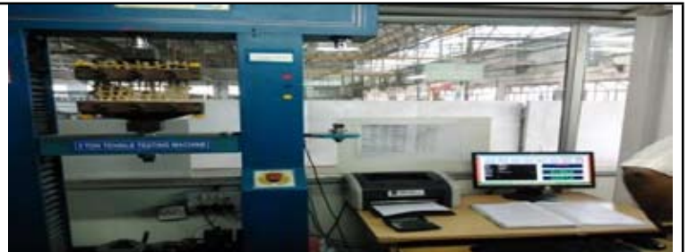
Fig. 10: Geomesh fitted into clamps with 50 mm grip on either side to make effective size of 200x100 mm for the test
