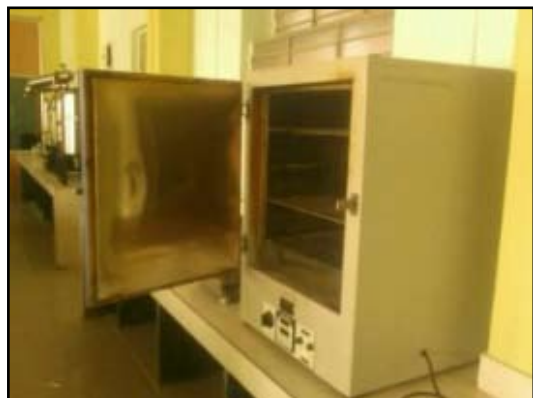
Fig. 6: Oven Dry Technique used for Gravimetric Method
