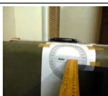
Fig.4.2: sliding table inclined at 41.5° & connected to ref.-00
