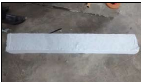
Fig 3 : External Wrapping by Geotextile
