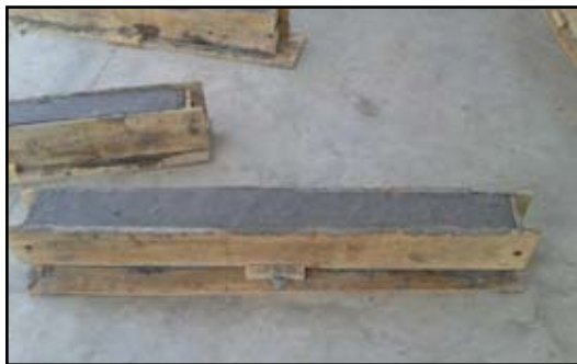
Fig 2 Formwork with Beam Specimen
