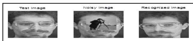
Fig.5: Nearest neighbor based Classification using Eigen face in case of Block Occlusion
