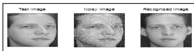
Fig.3: Nearest neighbor based Classification using Eigen face for Gaussian noise with variance 0.01
