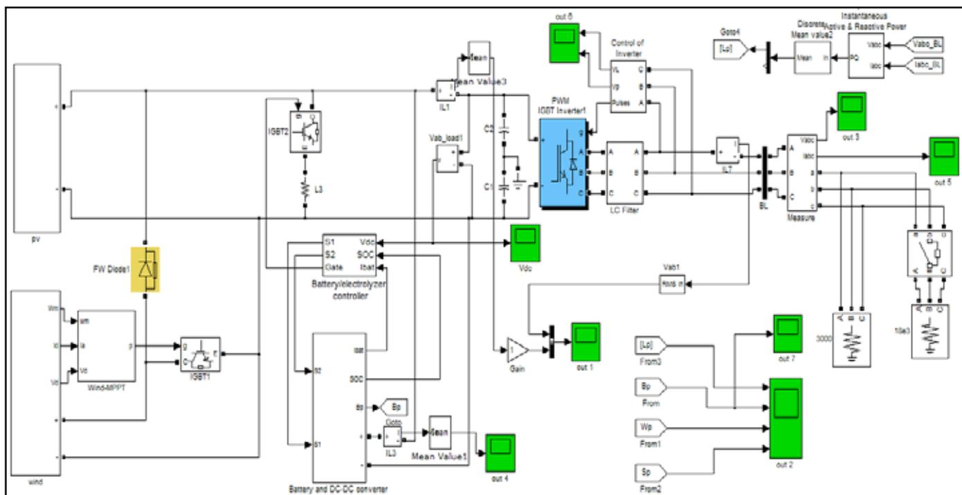
Fig. 5: Simulation diagram for Hybrid Wind-PV System
