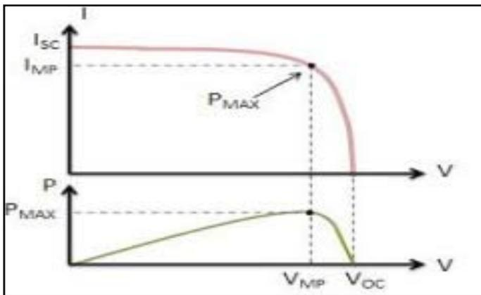
Fig. 4: Output characteristics of PV Array
