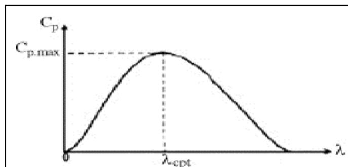
Fig. 2: Power coefficient vs Tip Speed Ratio
