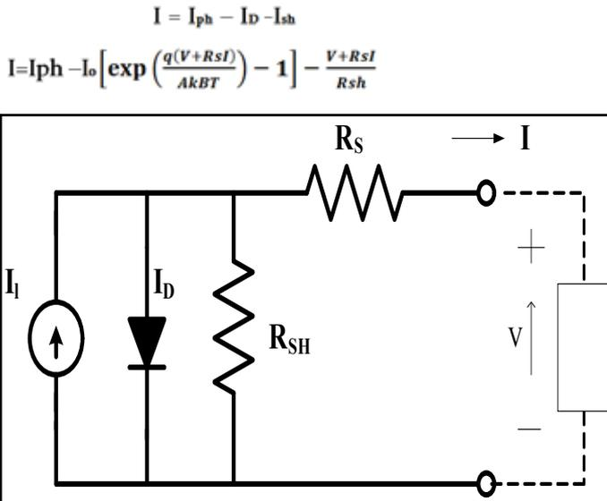
Figure 3: Equivalent circuit of PV Module
